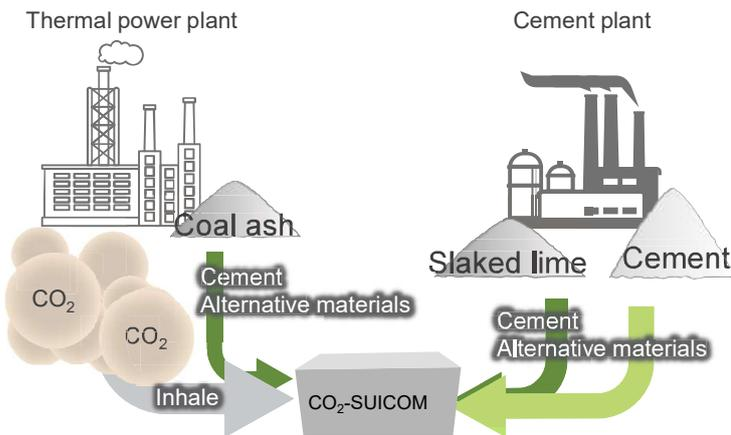
In "CO<sub>2</sub> - SUICOM", Reducing cement consumption by using coal ash, special admixtures and other materials instead of cement, and absorbing CO<sub>2</sub> into the concrete during manufacturing, we are able to reduce CO<sub>2</sub> emissions to virtually zero or less.
