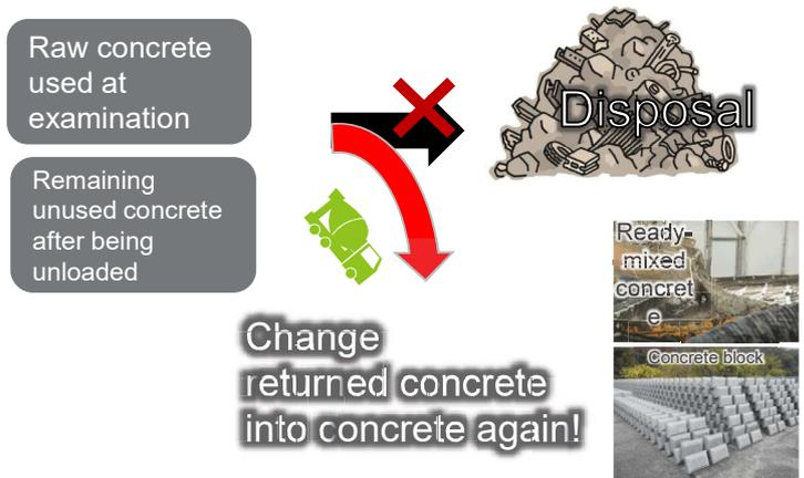
In "Eco-Crete R<sup>3</sup>", This is an environmentally conscious concrete that reuses the returned concrete which had been inevitably disposed. Eco-Crete contributes to resource recycling and reduce in CO<sub>2</sub> emissions.
